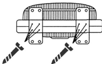
Install the supports using the screws provided
