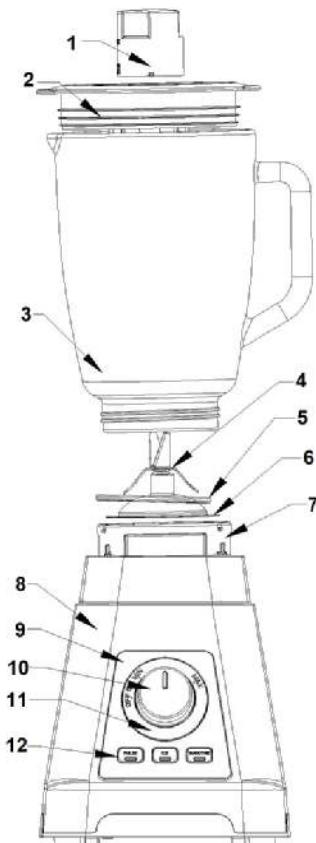
2. This unit have safety design, it do not work if the jar is not install on main body properly.
