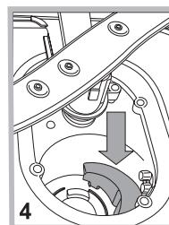
After cleaning the filters, re-place the filter assembly and fix it in position correctly; this is essential for maintaining the efficient operation of the dishwasher.
