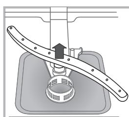
The lower sprayer arm can be removed by pressing on the side tabs and pulling it upwards.
