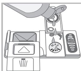
1. Open the dispenser "D" by pressing and pulling up the tab on the lid;
