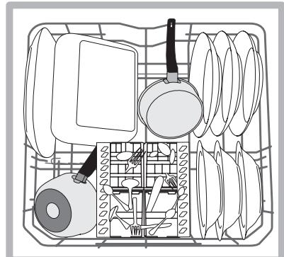
Very soiled dishes and pans should be placed in the lower rack because in this sector the water sprays are stronger and allow a higher washing performance.
