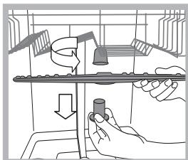
To remove the upper sprayer arm, turn the plastic locking ring in an anti-clockwise direction. The upper sprayer arm should be replaced so that the side with the greater number of holes is facing upwards.
