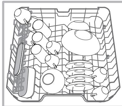
Several dishwasher models are fitted with tip-up sectors\*. They can be used in a vertical position when arranging tea/dessert saucers or in a lower position to load bowls and food containers.
