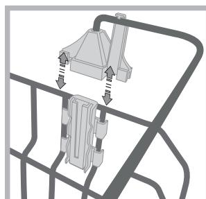
The upper rack can be adjusted for height based on requirements: high position to place bulky crockery in the lower rack and low position to make the most of the tip-up compartments/sectors by creating more space upwards.
