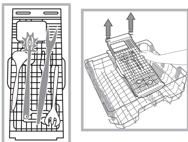
Before loading the tray, make sure the supports are properly coupled to the upper rack (*see Figure*).
