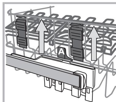
If the rack is equipped with a **Lift-Up device\*** (*see figure*), lift it up by holding its sides. To restore the lower position, press the levers (A) at the sides of the rack and follow the rack down.
