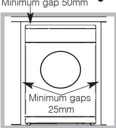
This is to ensure proper air circulation. Make sure that the back vents are not obstructed.
